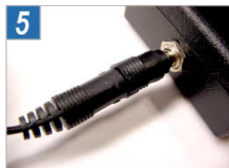
Step 5 – Attaching the Auxiliary Battery to the Solar Charger
